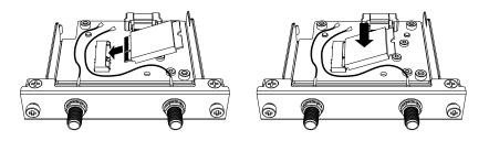
3. Secure the card with the screw removed in step 1.
