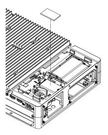
Put in the heat sink, and attach with screws.
