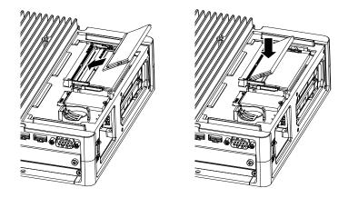
5. Replace the maintenance hatch cover and tighten the screws. **NOTE:** The necessary torque is 0.3 N•m (2.7 lb-in).
