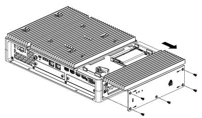
Insert the HDD or SSD into the slot.
