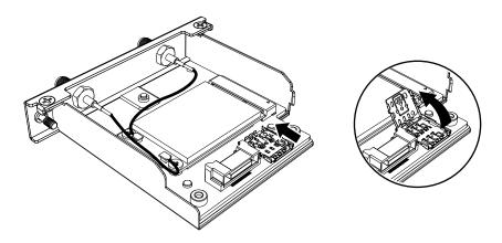
6. Insert the SIM card into the slot.
