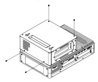
4. Slide the cover in the direction of the arrow on the top of the cover, and remove it.
