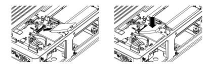
7. Secure the M.2 SSD card with the screw removed in step 5.
