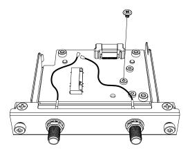
2. As shown below, insert the WiFi/Bluetooth card diagonally, then push from above.
