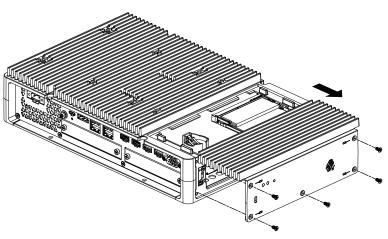
4. When equipped with M.2 SSD, remove the heat sink and heat sink pad (for top) before installing the FAN kit. For information on the heat sink and heat sink pad for M.2 SSD, see M.2 SSD Installation, page 97.
