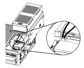
Using the screws removed in step 3, secure the FAN kit.
