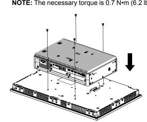
Tighten the M4 screws (4 pieces) to attach the Box Module.
