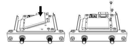
4. As shown below, plug the antenna cable connector securely to the connector on the 4G mini PCIe card. Looking from above the interface, plug the able connector on the left side to connector 1, and the cable connector on the right side to connector 2.
