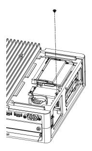
8. Peel off the protective film from the underside of the upper heat sink pad, and place the heat sink pad on the M.2 SSD card. Also peel off the protective film from the top surface of the heat sink pad. When using the Advanced Box with the FAN kit, this step is unnecessary.
