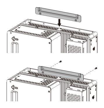
2. Install the product to the panel or wall with M4 screws (4 pieces).
