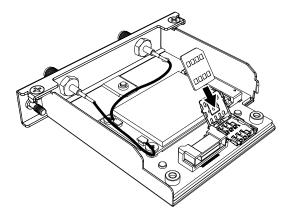
7. Close and slide the cover in the direction of the arrow to lock.
