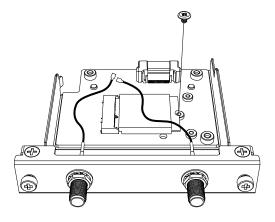
4. As shown below, plug the antenna cable connector securely to the connector on the card. Looking from above the interface, plug the cable connector on the left side to connector 1, and the cable connector on the right side to connector 2.
