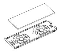
Re-insert the fan filter tray and tighten the screw.
