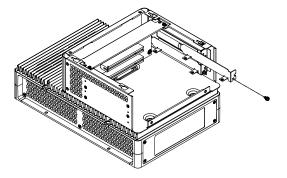
6. Insert the PCI/PCIe card, and secure the card with the screw removed in step 5.
