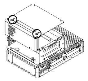
5. Remove the screw from the interface cover, then remove the cover.
