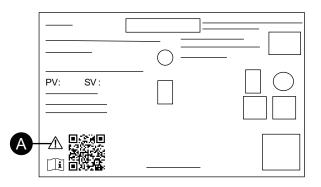
A. This mark indicates that you can refer to this manual by using the QR code, and that you must use copper wire rated for 75 °C (167 °F) or higher. Refer to Wiring the Power Supply, page 87.
