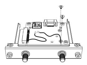
2. Connect the 4G mini PCIe card to slot.
