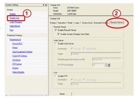
Check [Enable Remote Viewer] and [Enable Screen Changes from Client].
