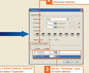
Right-click on a part with either a Switch Address, Interlock Address, or Lamp Address. Then select "Duplicate".
