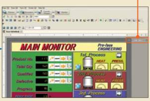
The 'Display Navigator' function is a default for Ver.2.5 or later. It's not necessary to set it in advance
