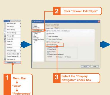
Display the overlapping parts by clicking [-/+] in the Display Navigator
