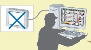
Simulate the environment of an HMI connected to a PLC to check the operation and debug projects on your PC.
