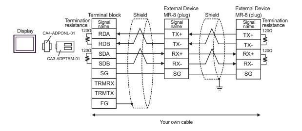
NOTE • When the External device has the SG terminal, connect it to the SG terminal of the Display.
