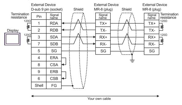
**NOTE** • When the External device has the SG terminal, connect it to the SG terminal of the Display.
