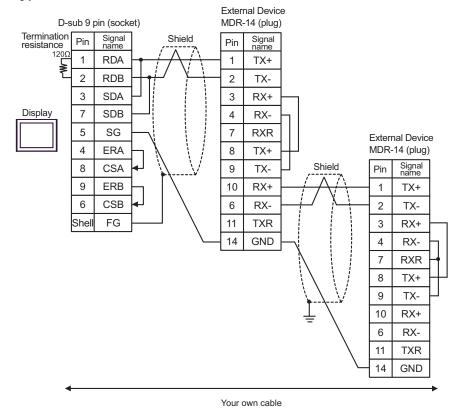
C) When using the online adapter (CA4-ADPONL-01), the terminal block conversion adapter (CA3-ADPTRM-01) by Pro-face and your own cable
