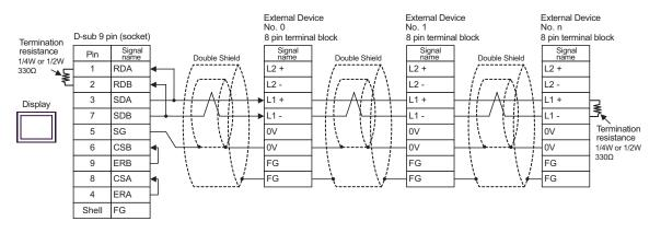
C) When using the online adapter (CA4-ADPONL-01), the terminal block conversion adapter (CA3-ADPTRM-01) by Pro-face, and your own cable
