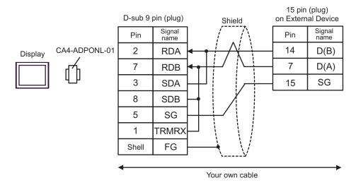
E) When using the COM port conversion adapter (CA3-ADPCOM-01), the connector terminal block conversion adapter (CA3-ADPTRM-01) by Pro-face and your own cable
