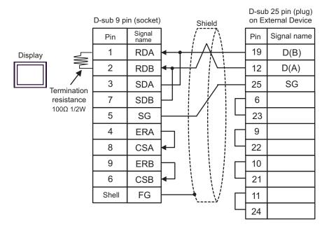
C) When using the online adapter (CA4-ADPONL-01), the connector terminal block conversion adapter (CA3-ADPTRM-01) by Pro-face and your own cable
