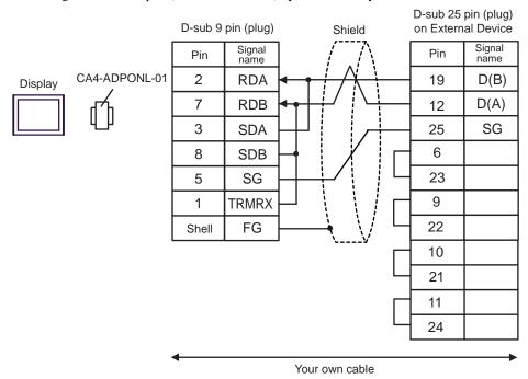
E) When using the COM port conversion adapter (CA3-ADPCOM-01), the connector terminal block conversion adapter (CA3-ADPTRM-01) by Pro-face and your own cable
