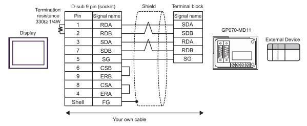
C) When using online adapter (CA4-ADPONL-01), 2-port adapter cable for AGP (CA3-MDCB11) by Pro-face and 2-port adapter II (GP070-MD11) by Pro-face.
