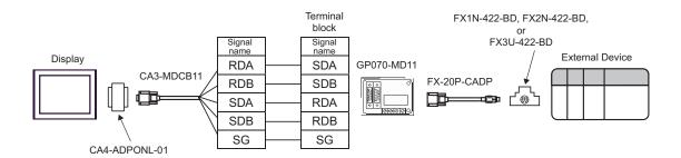
D) When using the online adapter (CA4-ADPONL-01) by Pro-face, your own cable, the 2-port adapter II (GP070-MD11) by Pro-face, the connector conversion cable (FX-20P-CADP) by Mitsubishi Electric Corp. and the function extension board (FX1N-422-BD, FX2N-422-BD or FX3U-422-BD) by Mitsubishi Electric Corp.
