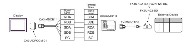
B) When using your own cable, the 2-port adapter II (GP070-MD11) by Pro-face, the connector conversion cable (FX-20P-CADP) by Mitsubishi Electric Corp., and the function extension board (FX1N-422-BD, FX2N-422-BD or FX3U-422-BD) by Mitsubishi Electric Corp.
