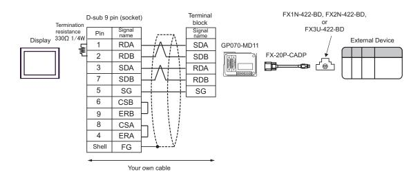
C) When using the online adapter (CA4-ADPONL-01) by Pro-face, the 2-port adapter cable for AGP (CA3-MDCB11) by Pro-face, the 2-port adapter II (GP070-MD11) by Pro-face, the connector conversion cable (FX-20P-CADP) by Mitsubishi Electric Corp. and the function extension board (FX1N-422-BD, FX2N-422-BD or FX3U-422-BD) by Mitsubishi Electric Corp.
