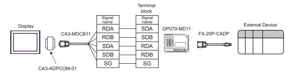
B) When using your own cable, the 2-port adapter II (GP070-MD11) by Pro-face and the connector conversion cable (FX-20P-CADP) by Mitsubishi Electric Corp.
