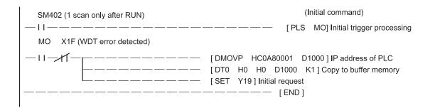
Above sample is the minimum ladder to enable UDP communication with AGP. Please refer to the manual of External Device for more information about error processing and TCP communication, etc.
