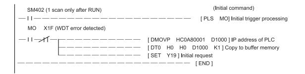
Above sample is the minimum ladder to enable UDP communication with Display. Please refer to the manual of External Device for more information about error processing and TCP communication, etc.
