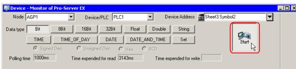
Device values are displayed according to the screen size with the specified device address (symbol) at the top.
