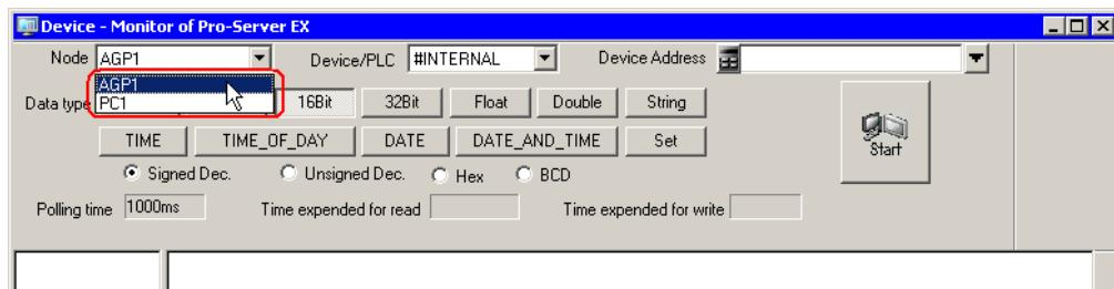
4 Click the list button of [Device/PLC] and select a Device/PLC having a monitoring device.
