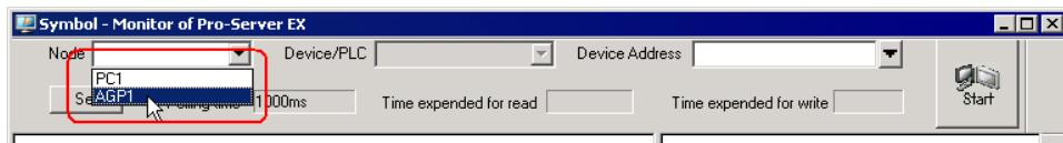
4 Click the list button of [Device/PLC] and select a Device/PLC having a monitoring device.
