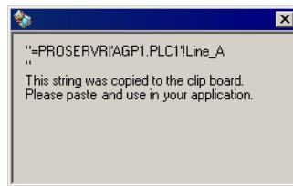
The DDE server uses information which consists of 3 parts, including [Application Name], [Topic Name], [Item Name] shown below, to communicate with an application.
