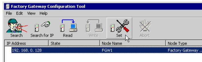
Protocol setup information of Device/PLC is read out, and the setup screen of communication protocol appears.
