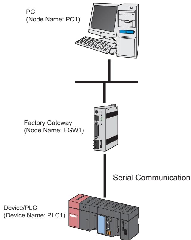
This section describes the setting procedures for making the above connection as an example.
