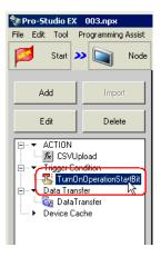
Specified data transfer and ACTION are now displayed on the "Sequence Diagram by Trigger Condition" screen.
