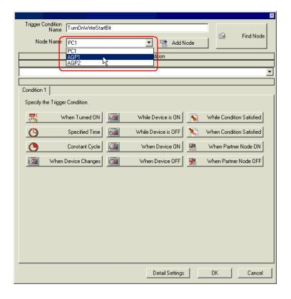
4 Click the [When Device On] button in the [Condition 1] tab, and select "PLC1" as a device name and then "Start Write" as a device symbol name to be a trigger. Then click the [OK] button.
