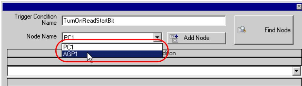
**NOTE** • Here, you are to specify the node having the device to be the trigger condition or having data to transfer.
