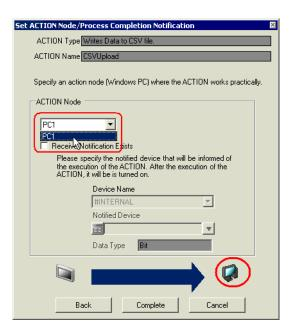
10 Turn off the check box of [Receive Notification Exists], if checked.
