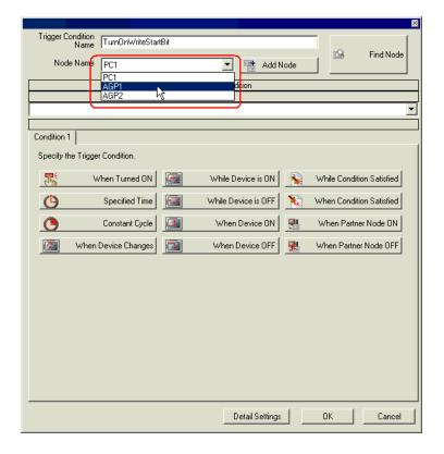
4 Click the [When Device On] button in the [Condition 1] tab, and select "PLC1" as a device name and then "Start Write" as a device symbol name to be a trigger. Then click the [OK] button.
