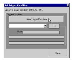
18) Enter the trigger condition name "Create a form" in [Trigger Condition Name], and select "AGP1" in [Node Name] as a name of the data transfer source.
