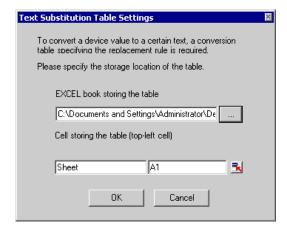
12) Enter the sheet name in [Cell storing the table]. Click the cell range specification button, and then enter the sheet name of the text substitution table and the cell number "A2" of the top-left cell.
