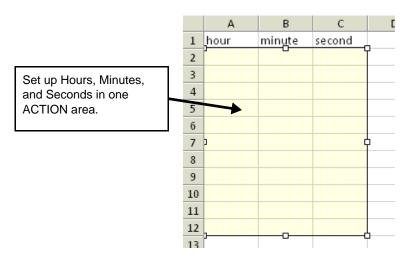
The above illustration shows the ACTION area that gets the Hours, Minutes, and Seconds from the external device's clock register, and populates the data in columns A, B, and C. Columns A, B, and C are set up in a single ACTION area. In the [Execution Sequence List] screen, set up one trigger condition to run one ACTION area.
