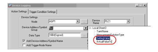
5) Turn off the [Add Device Address/Symbol Name] check box, if checked.
