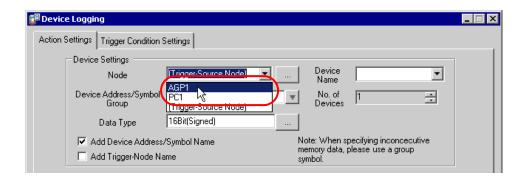
3) Click the list button of [Device Name] and select "PLC1" as a data transfer source device.
