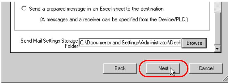
This is the end of setting an ACTION item necessary for mail send. The screen that explains the procedures to follow (saving and transferring network project file) will appear.
