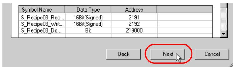
This is the end of registering symbols necessary for data write. The trigger condition setting screen will appear.
