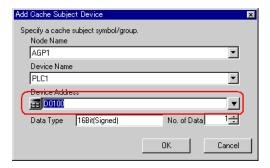
5) Set "16Bit(Signed)" in [Data Type] as a device data type and "1" in [No. of Data] as the number of devices, then click the [OK] button.
