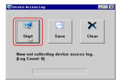
Collection of device access logs starts with the [Now collecting device access log] message displayed.
