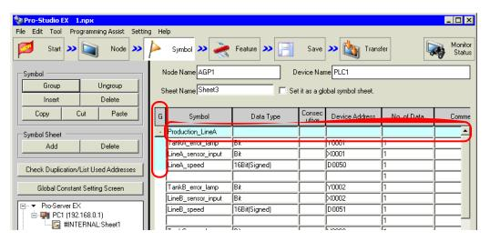
With the group configuration symbols displayed, the [-] button is placed in the column displaying the group name. Clicking the [-] button hides the configuration symbols and displays only the group name. (The [-] button changes to the [+] button.)
