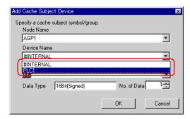
4) Set "D100" in [Device Address] as a device to be cached.
