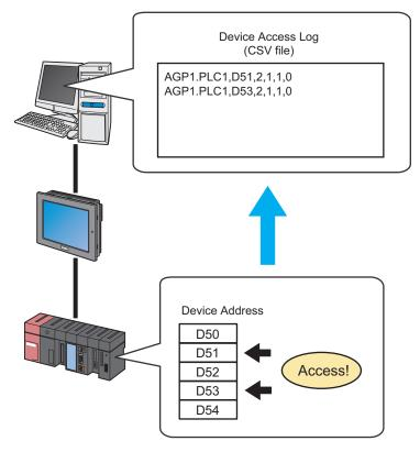
This section describes a series of actions to collect, save and clear device access logs.
