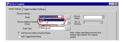
3) Click the list button of [Node] and select "PLC1" as a data transfer source device.
