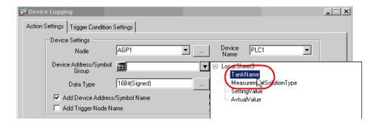
The device number "1" will be automatically entered in [No. of Devices], and "16Bit(Signed)" in [Data Type].
