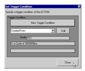
21) In [Logging], click the blank line of [Trigger Condition] and select "CreateAForm" as a trigger condition.
