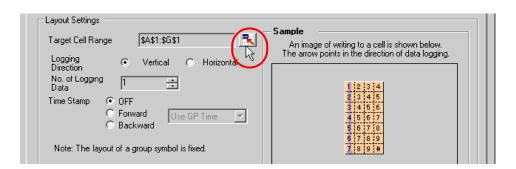
7) Drag the mouse to specify the area to use for data logging (cells B4 to C23). Then click the [OK] button.
