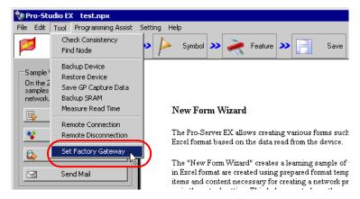
The Factory Gateway Configuration Tool starts.
