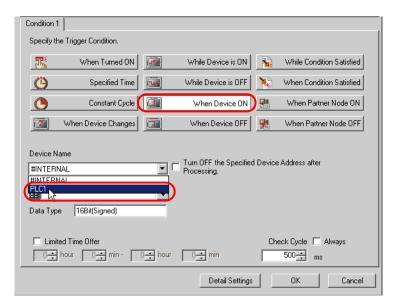
5 Click the [Device Address] list button and select "StartRead" for the symbol name of the device which serves as the trigger.
