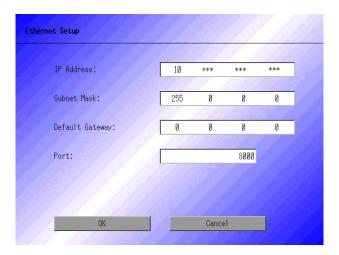
**3** Enter the numbers of the IP address, Subnet Mask, Default Gateway and Self Node, and then touch the [Set] button.
