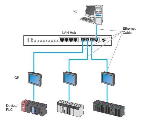
1 Connect one end of the Ethernet cable to the Ethernet port of the PC.
