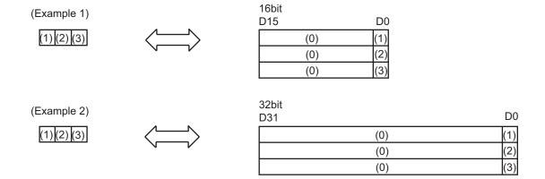
2) In the case of transferring data using the group symbol with the following structure (A combination of bit symbol, word symbol and bit symbol; the number of data of which are 1, 1, and 3, respectively).
