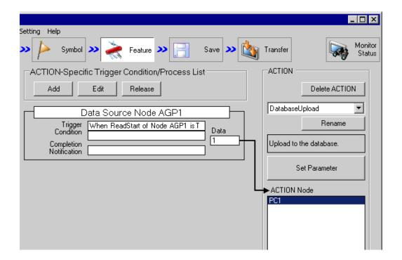
${\bf 2} \ \ {\bf Select the trigger condition name "TurnOnReadStartBit" from the tree display on the left of the screen.}$
