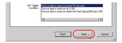
This is the end of setting a trigger condition necessary for data logging. The ACTION setting screen will appear.
