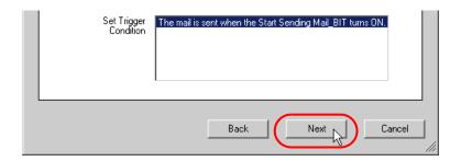
This is the end of setting a trigger condition necessary for mail send. The ACTION setting screen will appear.
