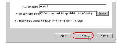
This is the end of setting an ACTION item necessary for data write. The screen that explains the procedures to follow (saving and transferring network project file) will appear. You can read the explanations how to save and transfer the network project file on the screen.
