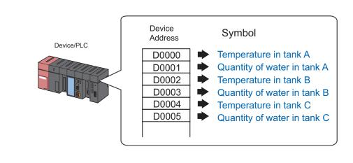
1 Check the [The symbols will be registered as data-source-node symbols.] check box, and then enlarge or scroll the screen to confirm the preset symbol.
