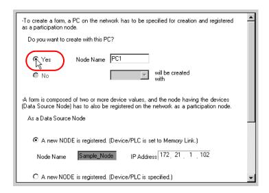
The PC currently used is set as an "Action Node", named as "PC1".
