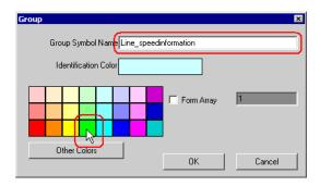
4 Check the [Form Array] check box, and enter the number of array (elements).
