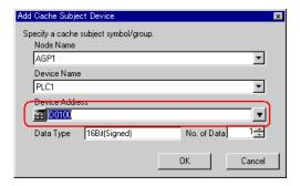
5) Set "16Bit(Signed)" in [Data Type] as a device data type and "1" in [No. of Data] as the number of devices, then click the [OK] button.
