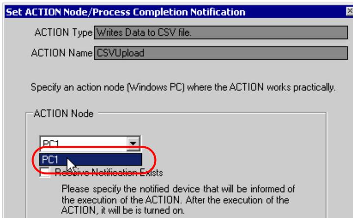
**NOTE** • When "Receive Notification Exists" is turned on, the specified bit device will be turned on when the ACTION is completed. This can be used as a trigger condition (trigger) of the subsequent ACTION when you want to execute two or more ACTIONS sequentially.
