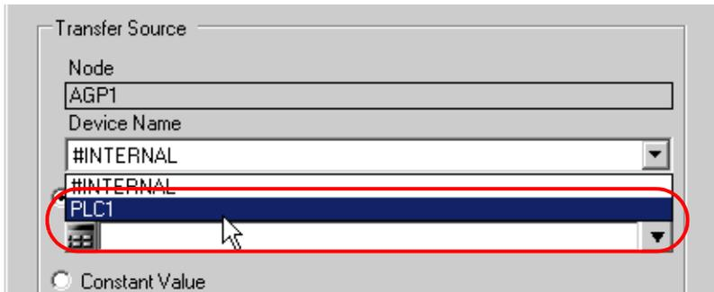
3 Click [Device Address] and then the list button to select "PLC1 data" for the symbol name of the Device/PLC "PLC1" reading data from.
