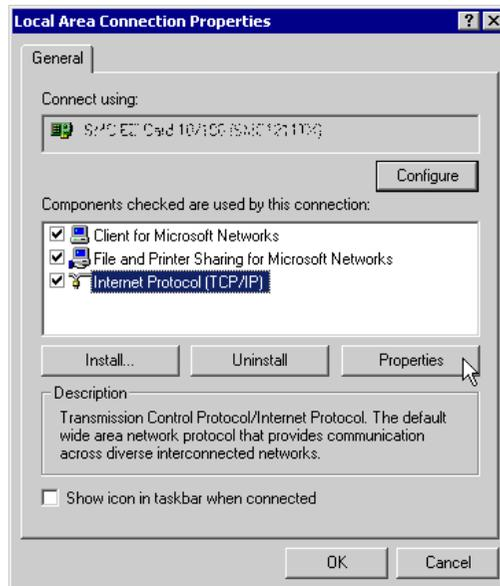
(5) In the "Internet Protocol (TCP/IP) Properties" dialogue, select [Use the following IP address], and then enter the IP address of the PC into the [IP address] field.
