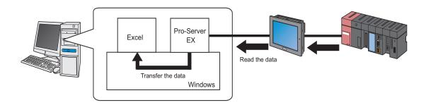
(5) 'Excel' displays the transferred data on the specified cell.
