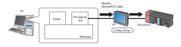
(2) The 'Pro-Server EX' notifies 'Excel' of a change in the data in the Device/PLC, if any.
