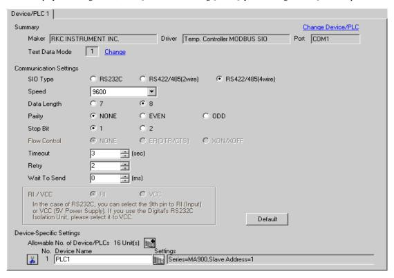
To display the setting screen, click [[Setting]] of the External Device you want to set from [Device-Specific Settings] of [Device/PLC Settings].
