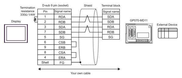
B) When using your own cable and 2-port adapter II (GP070-MD11) by Pro-face.
