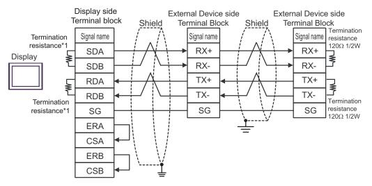
\*1 The resistance in the Display is used as the termination resistance. Set the value of the DIP Switch on the rear of the Display as shown in the table below.
