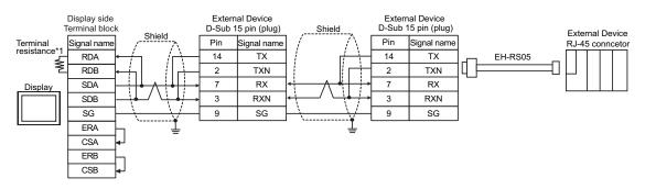
\*1 The resistance in the Display is used as the termination resistance. Set the value of the DIP Switch on the rear of the Display as shown in the table below.
