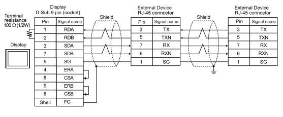
**NOTE** • Please turn on the DIP Switch 1 to enable build-in resistance(100 $\Omega$ ) on the remotest External Device side.
