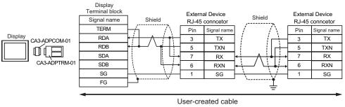
**NOTE** • Please turn on the DIP Switch 1 to enable build-in resistance( $100\Omega$ ) on the remotest External Device side.
