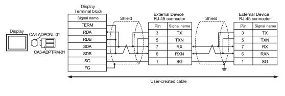
• Please turn on the DIP Switch 1 to enable build-in resistance( $100\Omega$ ) on the remotest External Device side.
