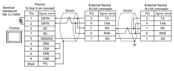
• Please turn on the DIP Switch 1 to enable build-in resistance(100 $\Omega$ ) on the remotest External Device side.
