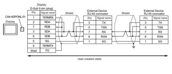
• Please turn on the DIP Switch 1 to enable build-in resistance(100 $\Omega$ ) on the remotest External Device side.
