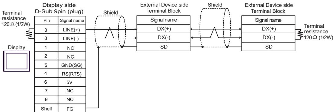
**IMPORTANT** • The 5V output (Pin #6) on the GP-4107 is the power for the Siemens AG's PROFIBUS connector. Do not use it for other devices.
