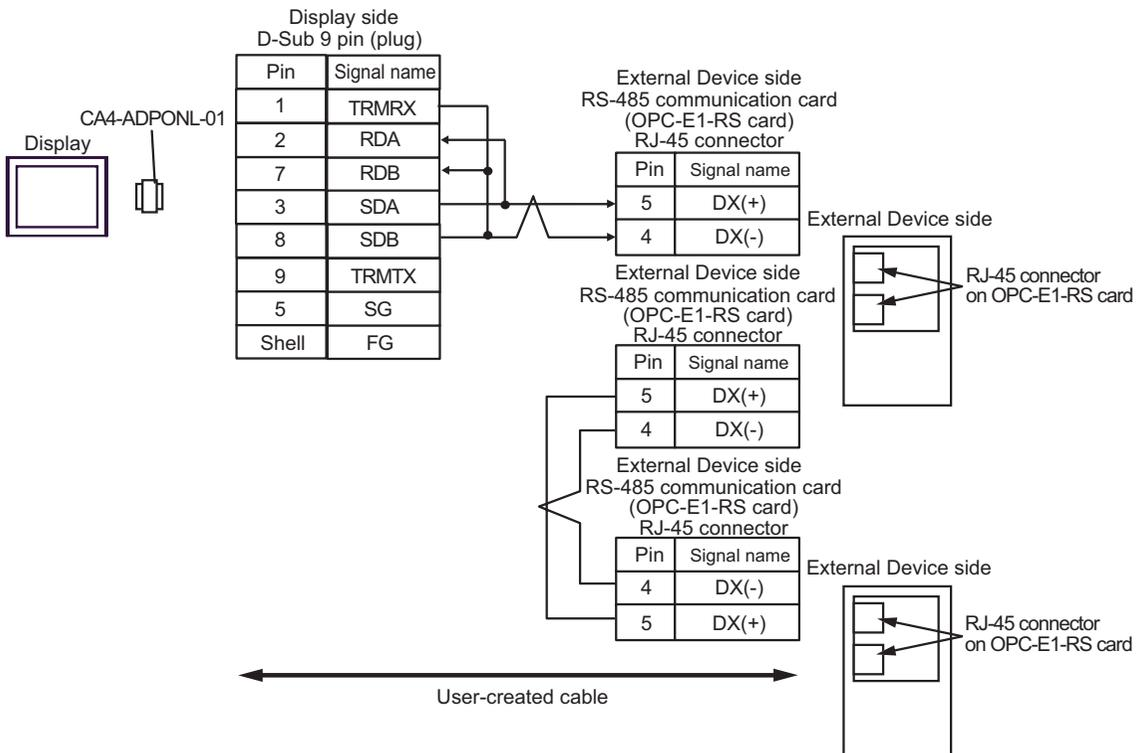
**NOTE** • For 1:n connection, set the termination resistance switch on the External Device located at the end to ON.
