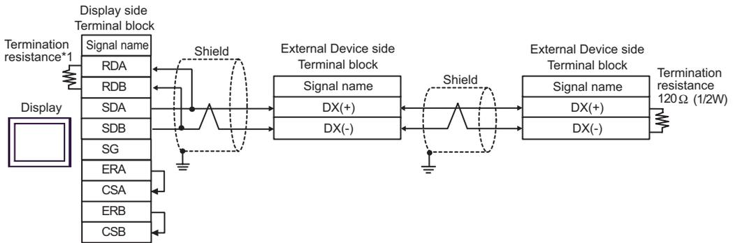
\*1 The resistance in the Display is used as the termination resistance. Set the value of the DIP Switch on the rear of the Display as shown in the table below.
