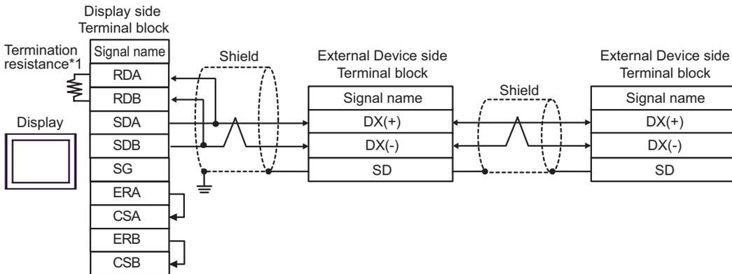
**NOTE** • For 1:n connection, set the termination resistance switch on the External Device located at the end to ON.
