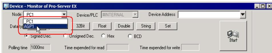
4 Click the list button of [Device/PLC] and select a Device/PLC having a monitoring device.
