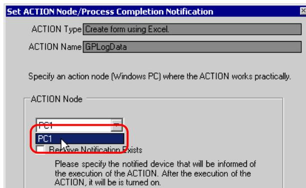
3 Turn off the check box of [Receive Notification Exists], if checked.
