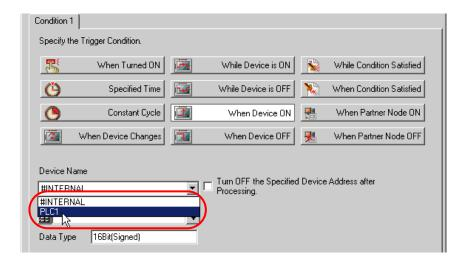
6) Click the [Device Address] list button and select "Start writing" for the device symbol name which serves as a trigger.
