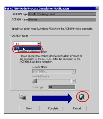
${\bf 3}$  Turn off the check box of [Receive Notification Exists], if checked.
