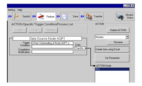
2 Select the trigger condition name "TurnOnReadStartBit" from the tree display on the left of the screen.
