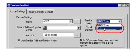
4) Click the list button of [Device Address/Symbol Group] and select "PLC1 data" as a symbol of the data to read out.
