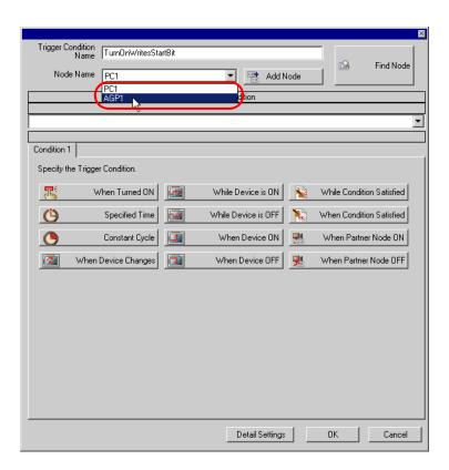
5) Click the [When Device ON] button in the [Condition 1] tab and select "PLC1" for the device name.
