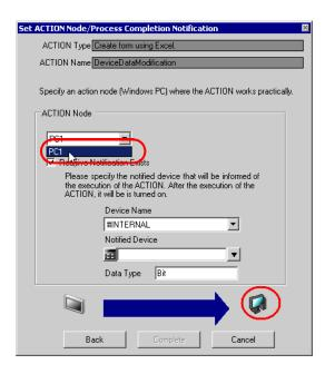
3 Turn off the check box of [Receive Notification Exists], if checked.
