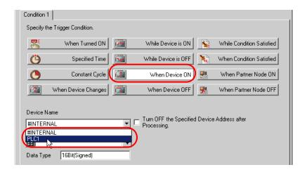
6) Click the [Device Address] list button and select "Start reading" for the device symbol name which serves as a trigger.
