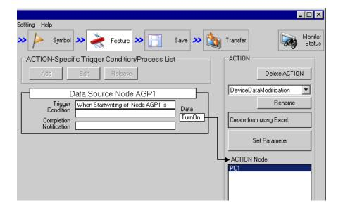
${\bf 2} \ \ {\bf Select the trigger condition name "TurnOnWritesStartBit" from the tree display on the left of the screen.}$
