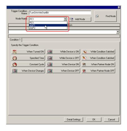
4 Click the [At Device On] button in the [Condition 1] tab, and select "PLC1" as a device name and then "Start write" as a device symbol name to be a trigger. Then click the [OK] button.
