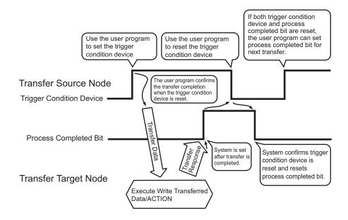
The following chart describes the summary of the rigger condition device, [Bit Showing Completion of the Process], [Bit Showing Processing Result (Success/Failure)], [Error Code Storage Location], [Abnormal Device IP Address Storage Location] and the timing to set the receipt notification device described later.
