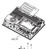
(4) Remove the IDE cover and plug the HDD unit cable connector in the IDE's interface (Seen the figure on the left).
