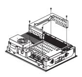
(3) Unscrew the screws (4), which are seen on the left figure, and remove the Expansion Board Base.
