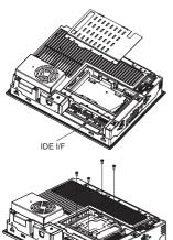
(4) Remove the IDE cover and plug the HDD unit cable connector in the IDE's interface (Seen the figure on the left).
