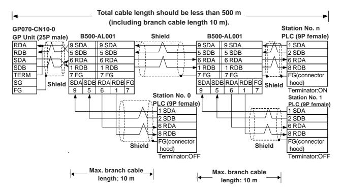
• When using Digital's RS-422 cable GP230-IS11-O
