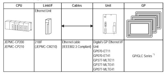
\*1 When using GP/GLC and the optional Ethernet I/F unit, refer to the following List of Connectable GP/GLC Units.
