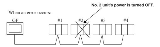
When unit #2's power is turned OFF, a communication error will occur. After the error occurs, the GP unit's communication retries will begin.
