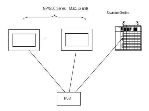
\* The maximum number of units indicated is when only GP units are connected. When other devices are connected via an ethernet connection, the number of GP units that can be connected is limited.
