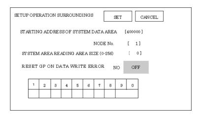
System area related and RESET GP ON DATA WRITE ERROR settings are performed via this screen. NODE No. indicates the PLC Node No. to which the system area has been allocated.
