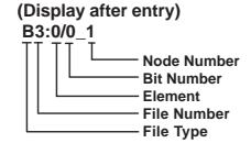
• When using Bit Devices T, C or R
