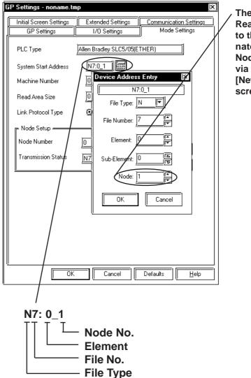
The System Area and Read Area are assigned to the PLC node designated here. Node Numbers are set via the [Mode Settings] -[Network Information] screen.
