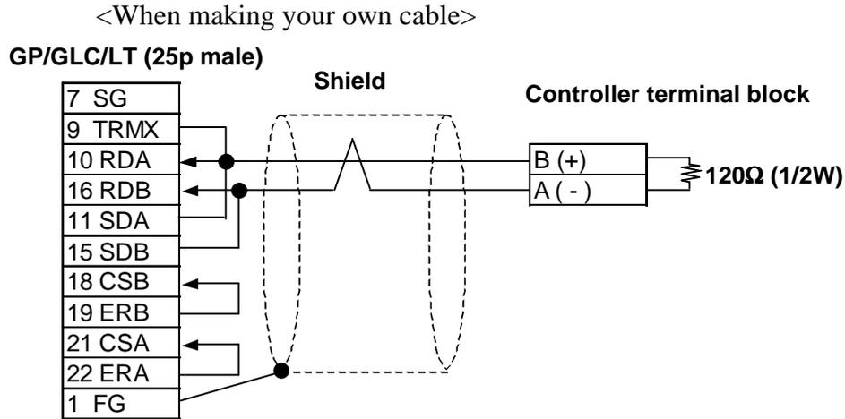
**Cable Diagram 3** (1:n) RS-422 2 Wires
