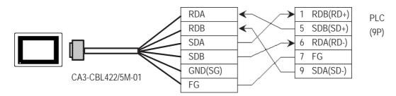
• When using Digital's RS-422 cable CA3-CBL422/5M-01
