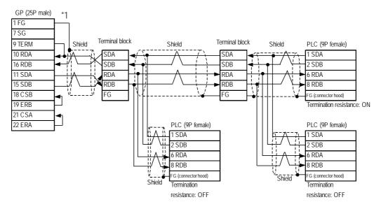
\*1 When connecting the #9 and #10 pins in the GP Serial I/F, a termination resistance of  $100\Omega$  is added between RDA and RDB.
