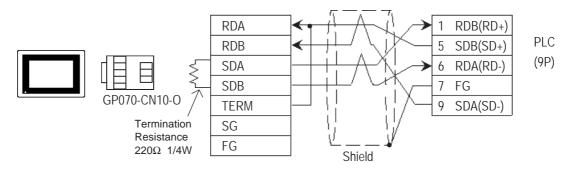
• When using Digital's RS-422 Cable, GP230-IS11-0
