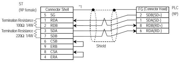
\*1 Be sure to connect the shield to the Connector Shell. For information about FG connections, refer to page 1-2 "RS422 I/F (ST400/ST403)" section's Note, in the "Connecting a Device/PLC to the ST unit."
