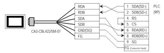
Be sure to connect the FG line to the FG terminal. For information about FG connections, refer to page 1-5 note \*1, in the "Connecting a Device/PLC to the ST unit."
