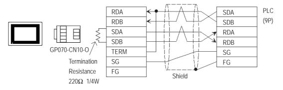
• When using Digital's RS-422 connector terminal adapter GP230-IS11-0
