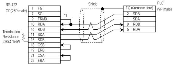
\*1 When connecting the #9 and #10 pins in the GP Serial I/F, a termination resistance of  $100\Omega$  is added between RDA and RDB.
