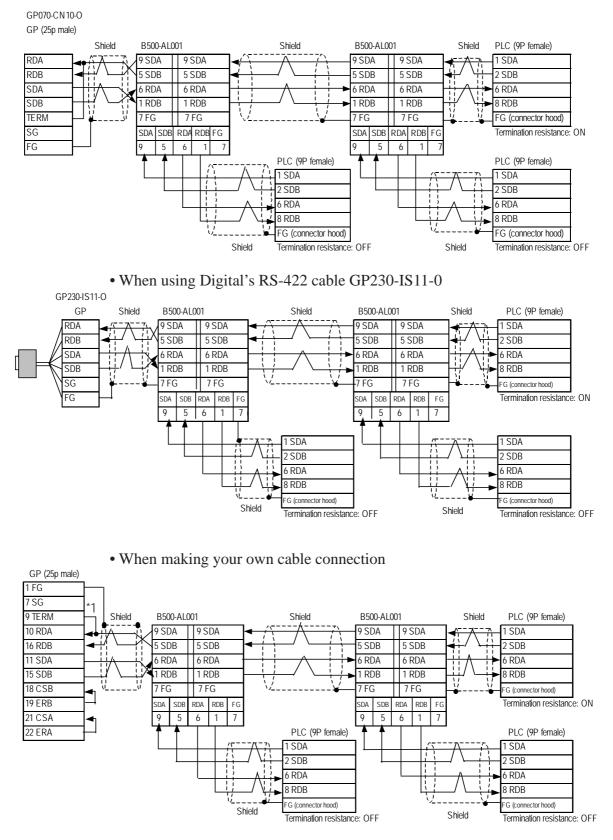
\*1 When connecting the #9 and #10 pins in the GP Serial I/F, a termination resistance of  $100\Omega$  is added between RDA and RDB.
