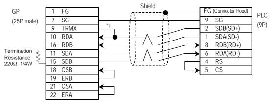
\*1 When connecting the #9 and #10 pins in the GP Serial I/F, a termination resistance of  $100\Omega$  is added between RDA and RDB.
