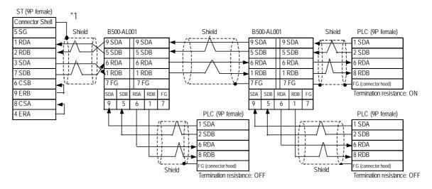
\*1 Be sure to connect the shield to the Connector Shell. For information about FG connections, refer to page 1-2 "RS422 I/F (ST400/ST403)" section's Note, in the "Connecting a Device/PLC to the ST unit."
