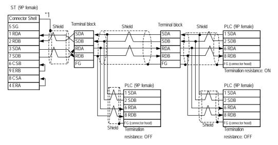
\*1 Be sure to connect the shield to the Connector Shell. For information about FG connections, refer to page 1-2 "RS422 I/F (ST400/ST403)" section's Note, in the "Connecting a Device/PLC to the ST unit."
