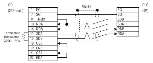
\*1 When connecting the #9 and #10 pins in the GP Serial I/F, a termination resistance of  $100\Omega$  is added between RDA and RDB.
