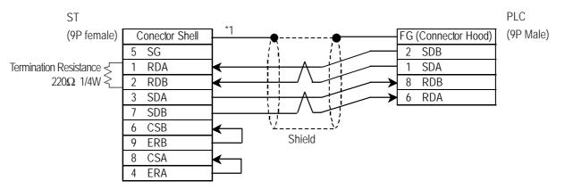
\*1 Be sure to connect the shield to the Connector Shell. For information about FG connections, refer to page 1-2 "RS422 I/F (ST400/ST403)" section's Note, in the "Connecting a Device/PLC to the ST unit."
