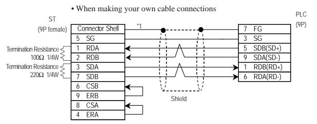
\*1 Be sure to connect the shield to the Connector Shell. For information about FG connections, refer to page 1-2 "RS422 I/F (ST400/ST403)" section's Note, in the "Connecting a Device/PLC to the ST unit."
