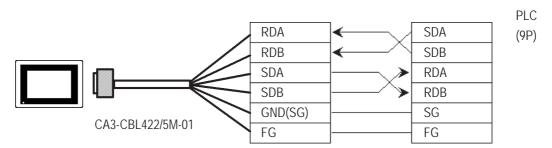
• When using Digital's RS-422 cable CA3-CBL422/5M-01
