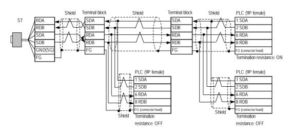
• When using Digital's RS-422 cable CA3-CBL422/5M-01
