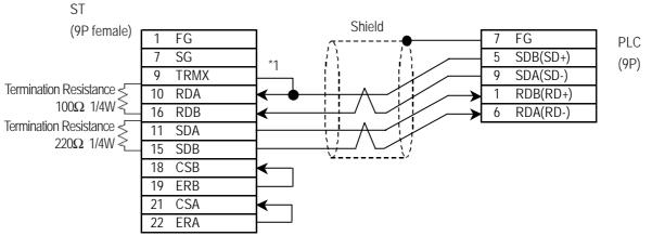
\*1 Be sure to connect the shield to the Connector Shell. For information about FG connections, refer to page 1-2 "RS422 I/F (ST400/ST403)" section's Note, in the "Connecting a Device/PLC to the ST unit."
