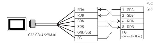
• When using Digital's RS-422 cable CA3-CBL422/5M-01
