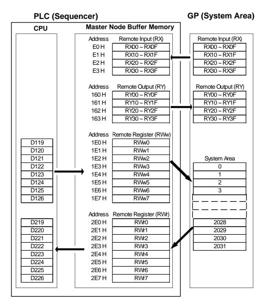
The figures show the PLC CPU's D119 used as the start address for the storage of commands, with D129 being used as the start address for the storage of read out data.
