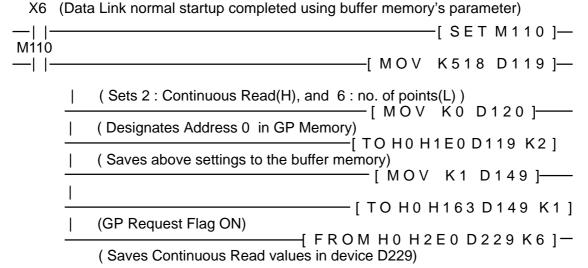
In order to send T-tag data to a PLC, and also enable the master station to read the touched value using the Continuous Read command.
