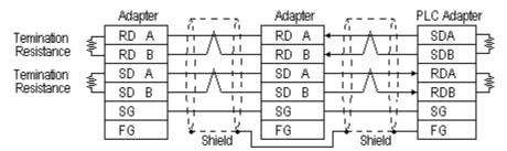
\* Check the PLC Adapter specifications for the Temination Resistance
