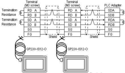
\*Check the PLC Adapter specifications for the Termination Resistance
