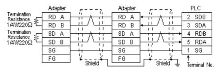
• When using Digital's Multi-link Cable, GP230-IS12-O
