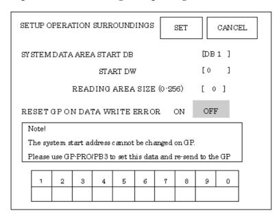
System Area related settings and On Data Write Error settings are performed via this menu. The system area start address cannot be changed via the GP unit. Be sure to use GP-PRO/PBIII Screen Editor software to change this data and resend it to the GP unit.
